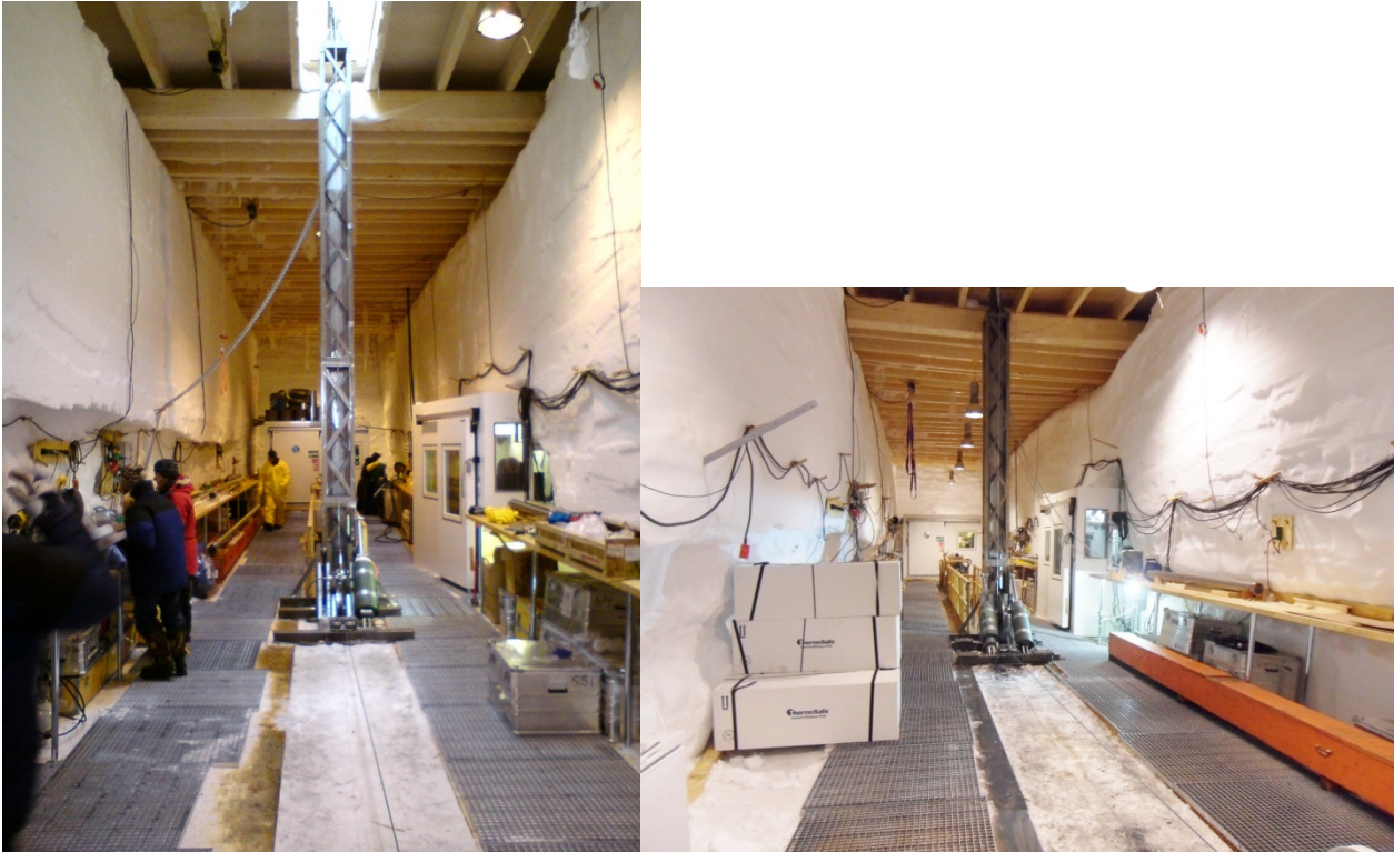
Left: NEEM drill trench June 2009. Right: NEEM drill trench June 2011. Notice the location of the top sheave in the slot in the roof. Between 2009 and 2011 the tower was shortened by 1.5 m (i.e. the section just above the foot of the tower was removed).
