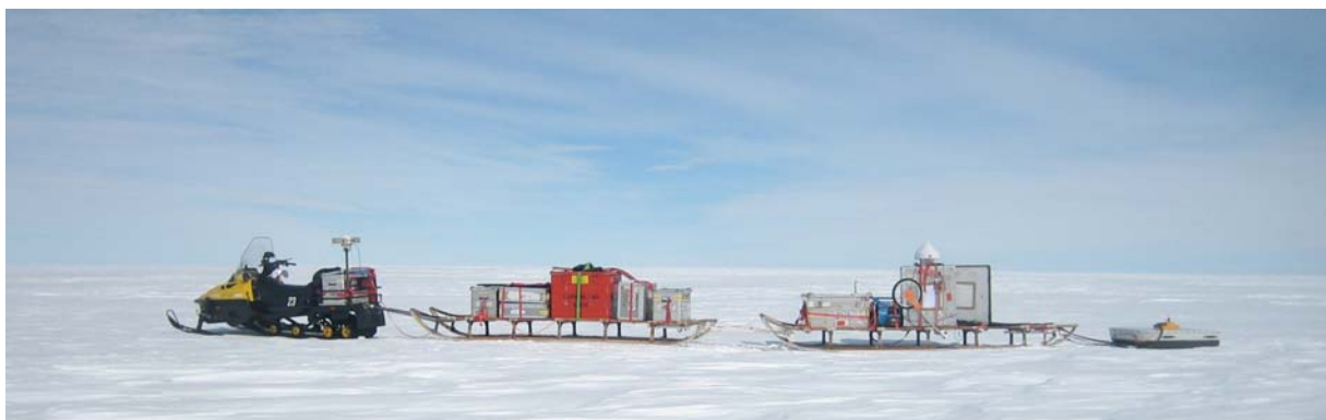
Figure: Example of the set-up of GPR and GPS equipment.
