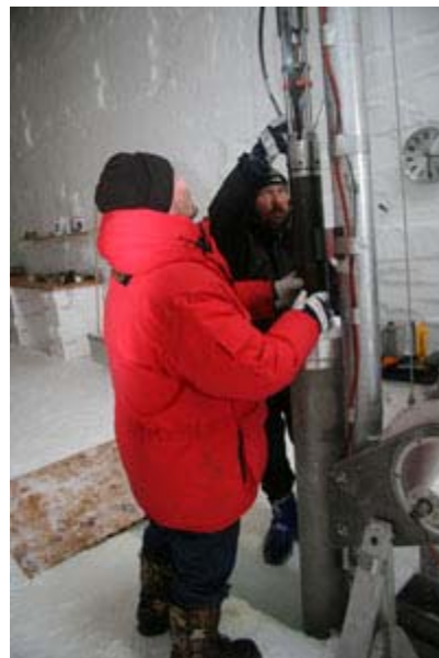
Reaming the borehole with the big reamer 5
