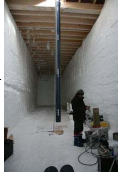
Casing the borehole
