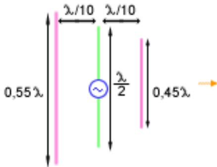
From left to right, the elements mounted on the boom are called,
