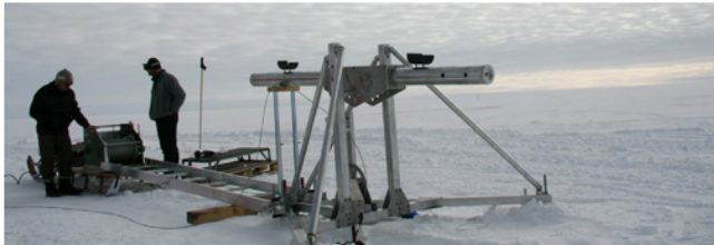
Simon and Henry getting the CH elevated tower and the DK intermediate winch together
