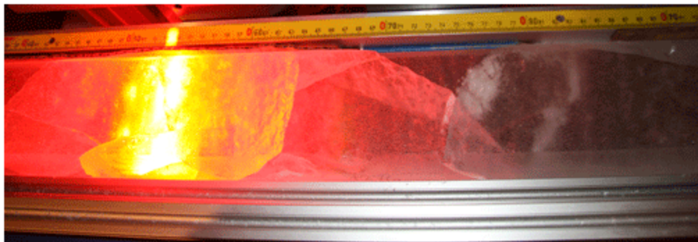
Brittle ice on fire in the line scanner. The internal breaks in the core are clearly visible.
