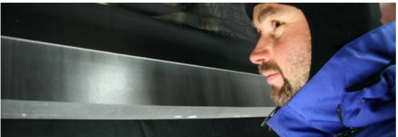
Gregory inspects the polished ice before it goes into the optical scanner.
