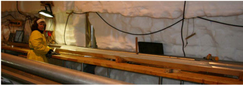
A 3.2 m long ice core from almost 2450 m depth is ready to be logged by Maggan. Such long cores of the warm ice at this depth are almost more than we can ask for.
