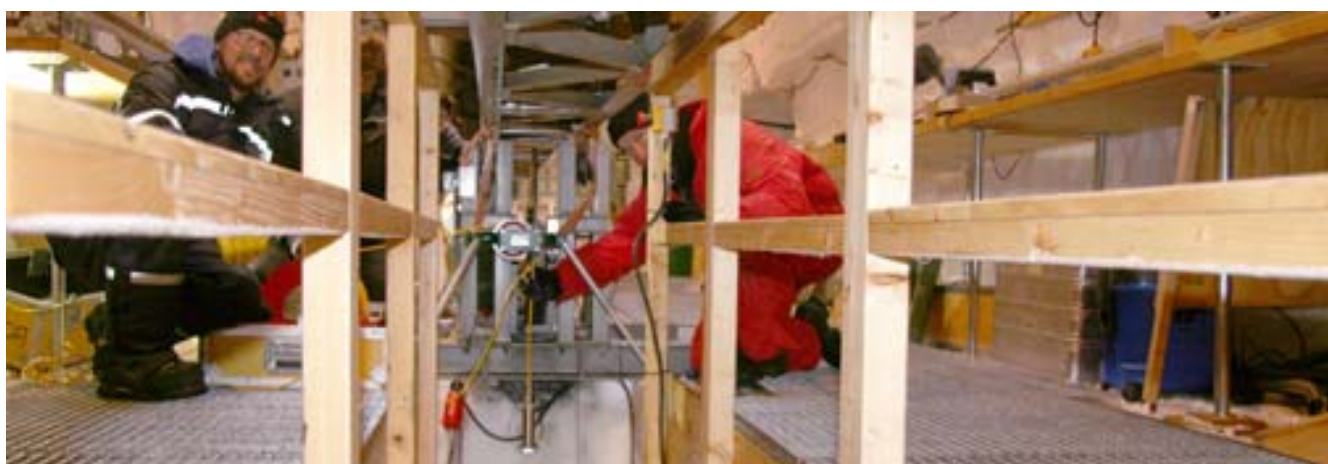
Trevor and Simon with the borehole camera. The camera is the small steel cylinder hanging from the cable.
