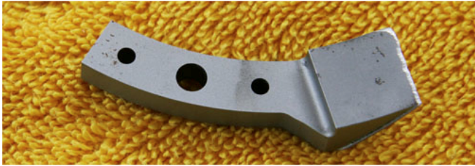
Destroyed ice drill cutter after drilling the ice with mud and pebbles.
