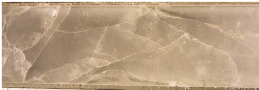
One of the worst pieces of brittle ice prepared with a microtoned surface before the ECM measurement
