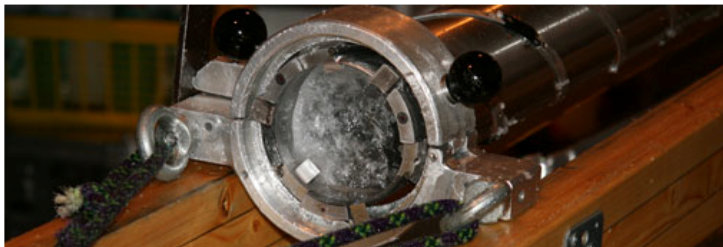
The core barrel with a freshly drilled core from 2444 m depth is pulled out of the drill. It appears that the ice crystals are smaller than they've been over the last weeks.
