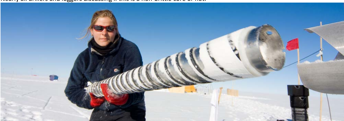
Anne pulling out the inner core barrel of the shallow drill at the firn-gas village.
