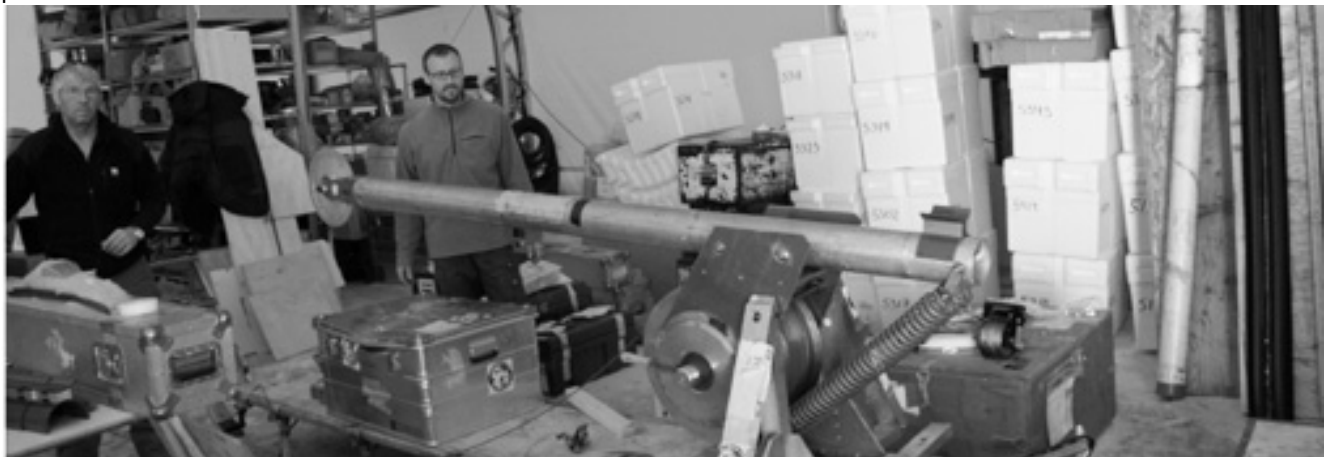
The shallow ice core drill is being assembled in the garage by Trevor and Sverrir. The shallow drill will be used to drill ice cores for several programs and the shallow borehole will be used for firn-gas measurements extending the big firn-gas program done last year at NEEM.
