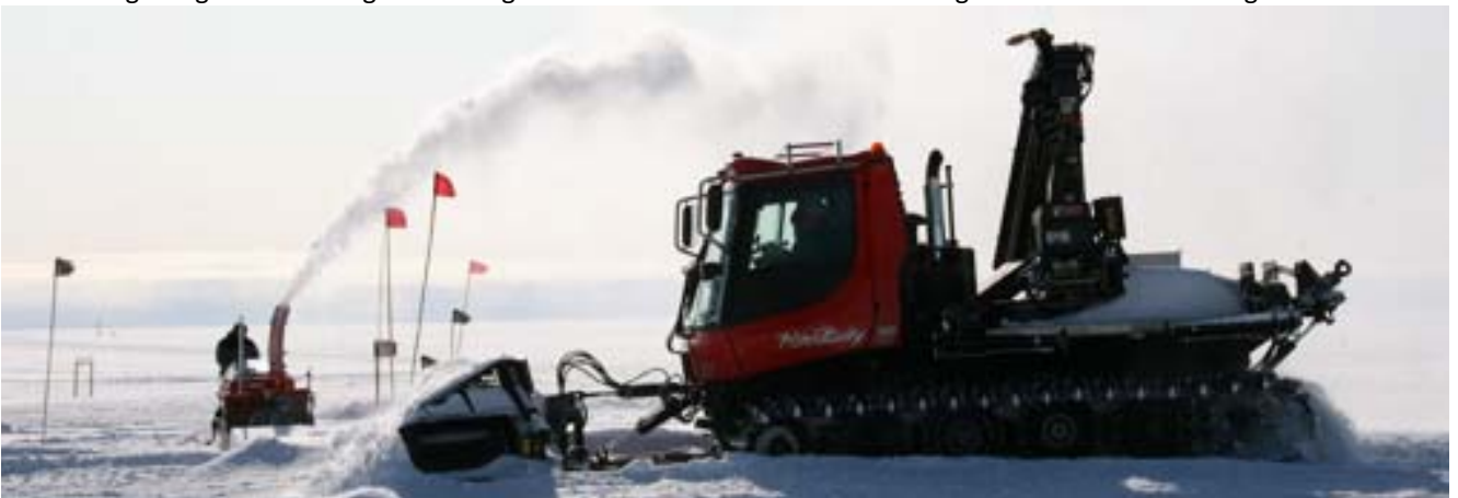
Active removal of snow around the main dome and the trenches: the snow blower on the roof of the science trench and the Pisten Bully between the main dome and the trench roofs.
