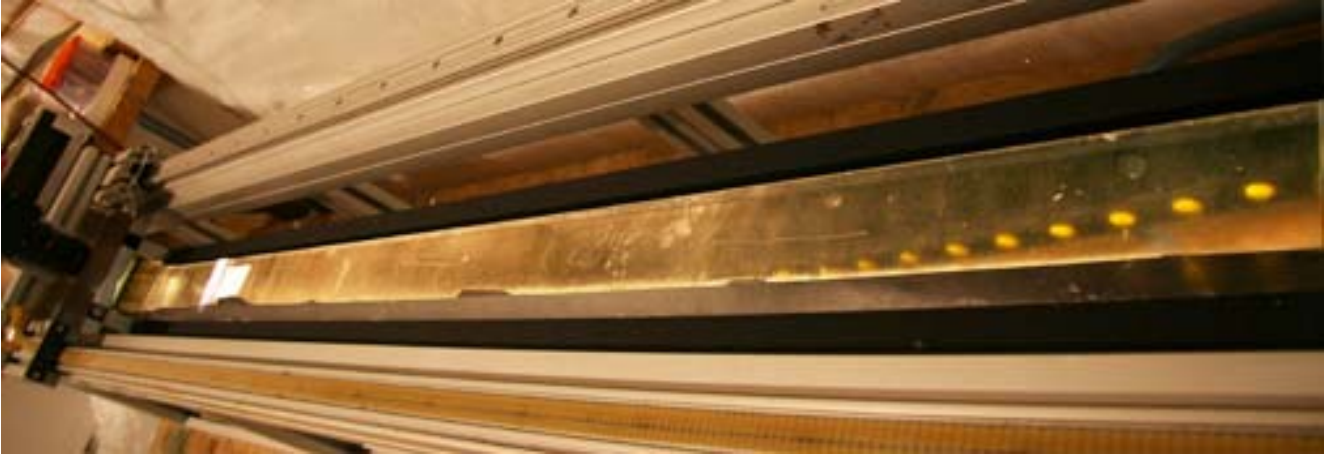
Figure caption: A 1.65m slab of ice in the line scan instrument in the science trench. The ice is in one piece with no breaks at all!
