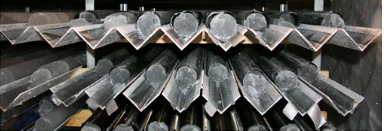
Brittle ice cores in the core buffer. The cores will be left in the core buffer over winter so they are less brittle when processed in the science trench.
