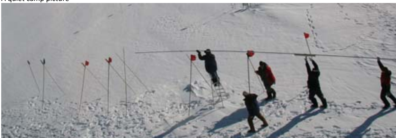
One of the attempts to improve the antenna was to try with an antenna of aluminum poles. The long aluminum, poles is placed above the surface on bamboo poles.
