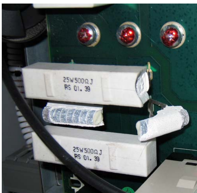
A piece of the broken part of the winch control.
