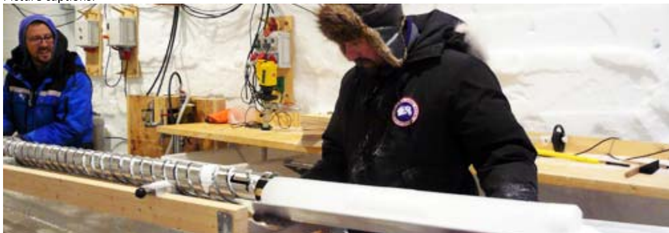
Trevor and Steff extract a 1 meter core from the HT drill.
