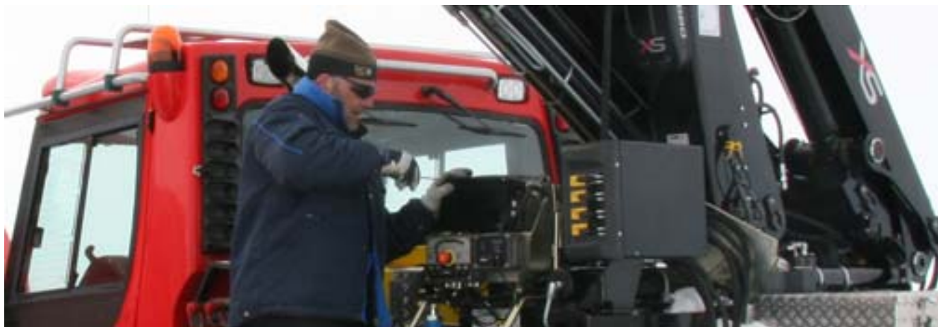
Caption: Gunnar doing maintenance of the Pistenbully crane control
