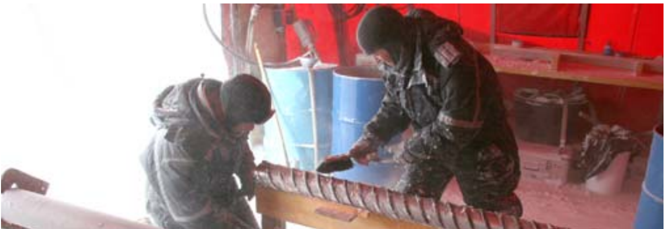
Darcyandandrew: Darcy and Andrew are trying to clean the core barrel in the blowing snow inside the storage garage.
