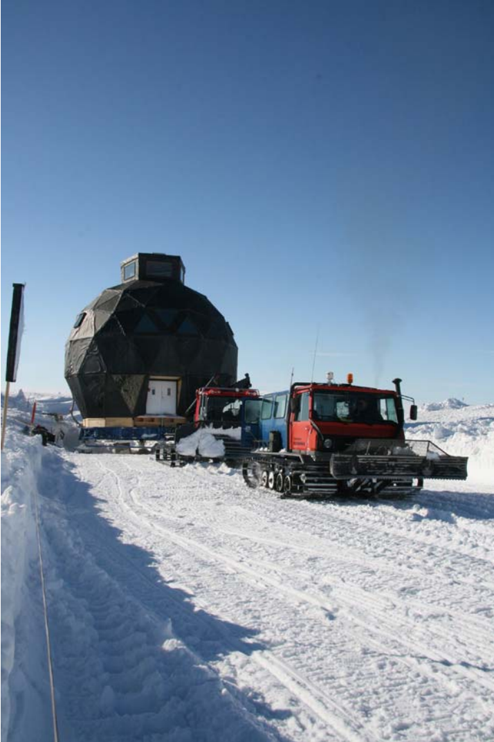
Dome being pulled by the Pisten Bully and Flexmobil
