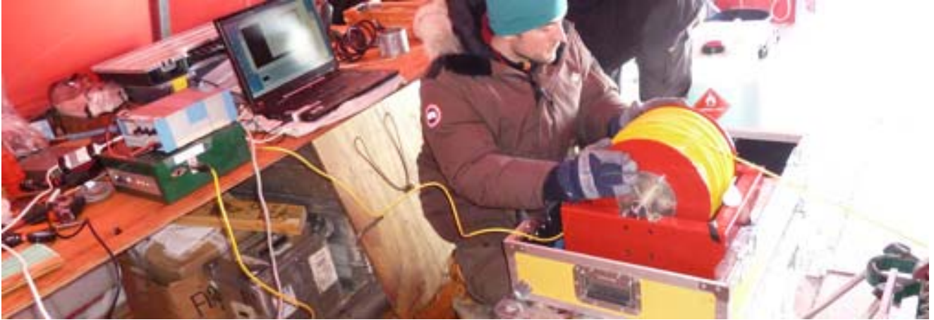
Christopher lowering the camera to view the replicate drilling progress
