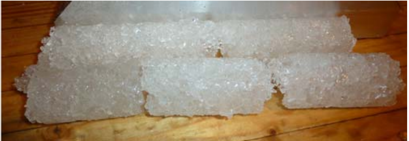
First core drilled with the 1 inch rock drill
