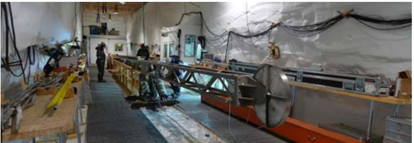
Tower: Inside the drill trench. The shortened drill tower is horizontal.
