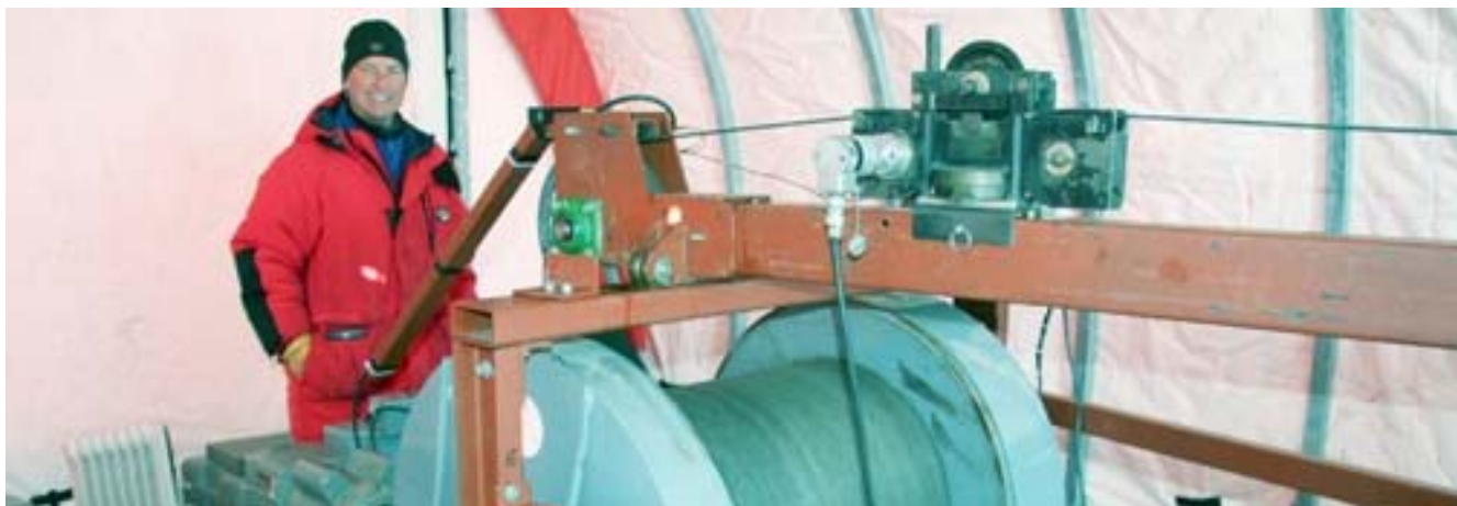
Gary: Gary at the best thermometer in Glaciology. He takes temperature readings with an absolute accuracy of 1 mK, all the way along the deep borehole.
