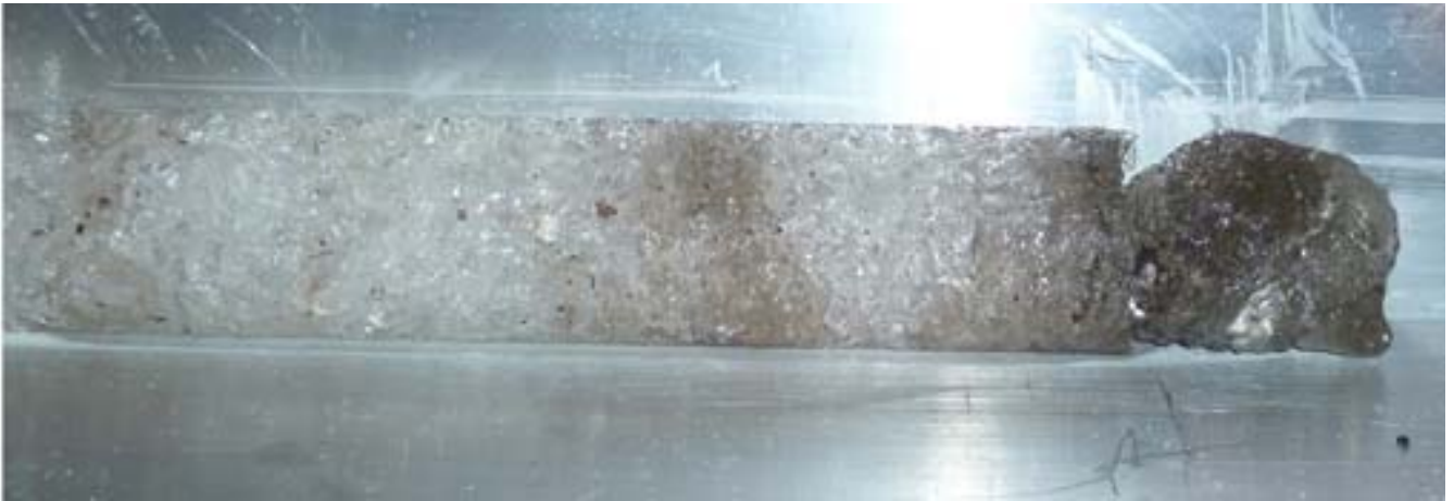
Second core drilled with the rock drill
