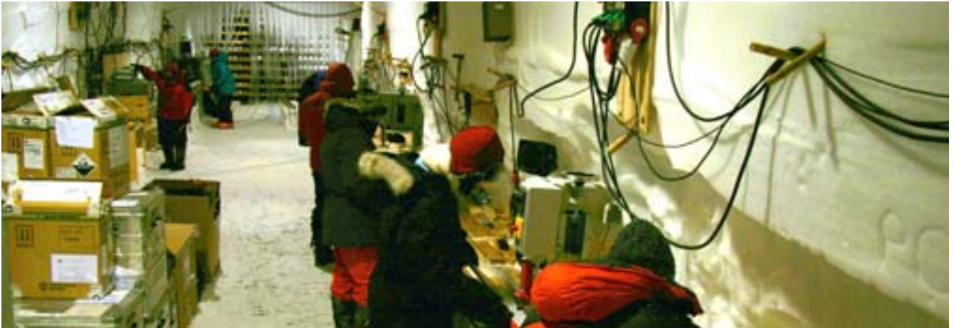
Science trench: Activity in the science trench. Here, people are performing electrical measurements on ice cores as well as cutting samples of various sizes. Finally, the remaining core and the samples are packed into crates and shipped to Europe, the U.S. and Asia.
