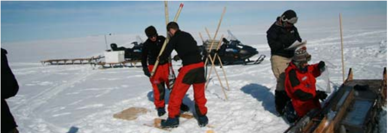
CFA team drilling firn cores a few km from the NEEM camp
