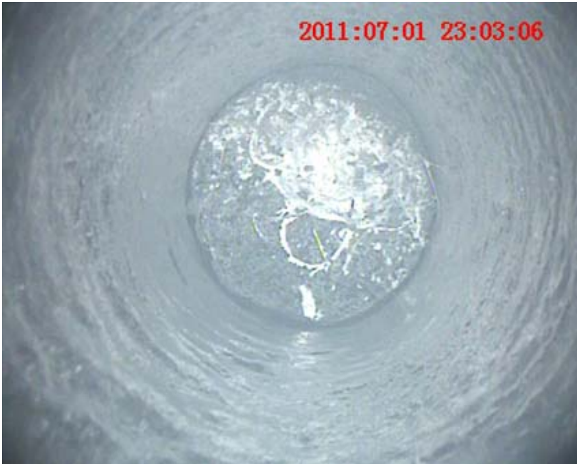
Picture of the bottom of the 2537m deep NEEM borehole.
