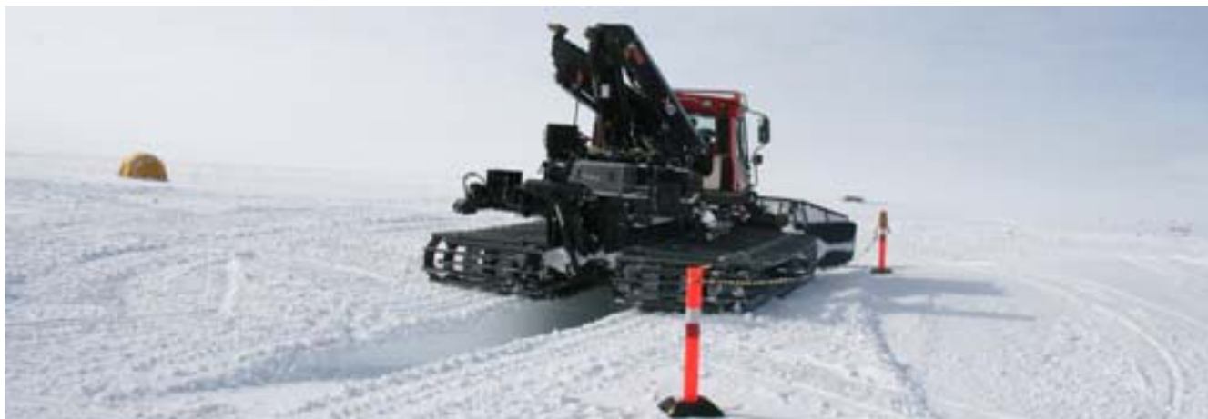
Pistenbully: The Pistenbully for service. A service trench has been made in the snow. All oil and spill is collected and sent to Kangerlussuaq of course.
