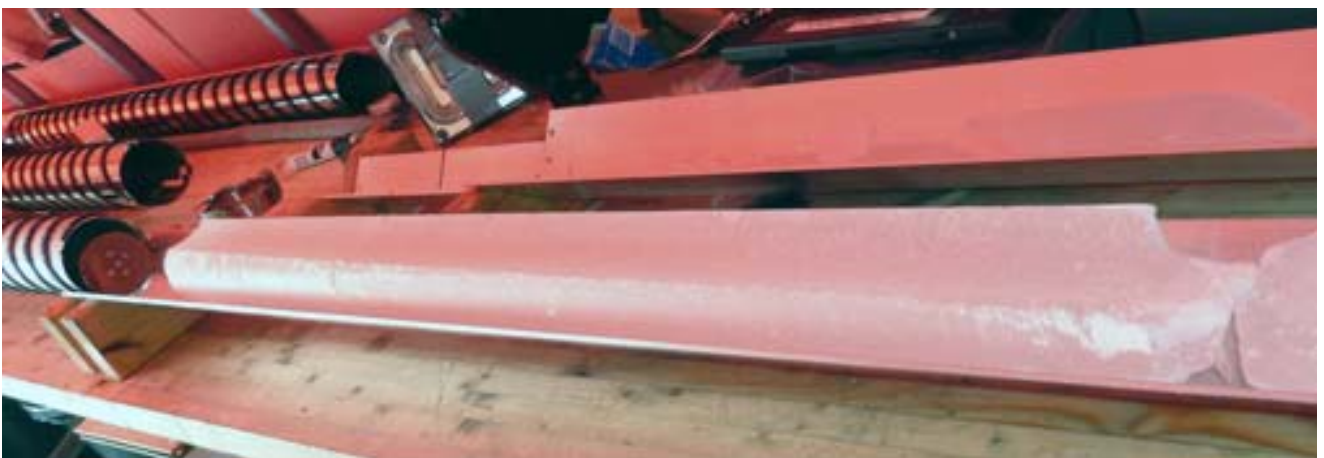
The first replicate core. The core gradually gains area as the drill pushes further and further out in the side wall of the original borehole.
